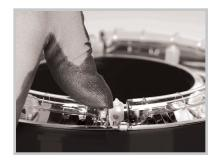
Each ABR800 unit employs a pair of half-circle flashtubes. Unless a single, half-circle flashtube has prematurely failed, it is best to replace both tubes at the same time.
